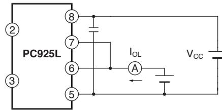
**Fig.3 Test Circuit for High Level Output Voltage**
