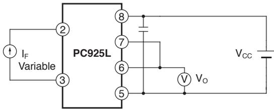
**Fig.8 Test Circuit for Response Time**
