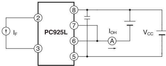
**Fig.2 Test Circuit for Low Level Output Current**
