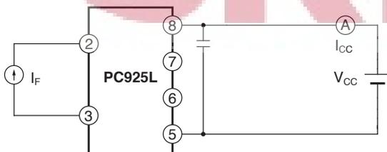
**Fig.6 Test Circuit for UVLO Threshold**
